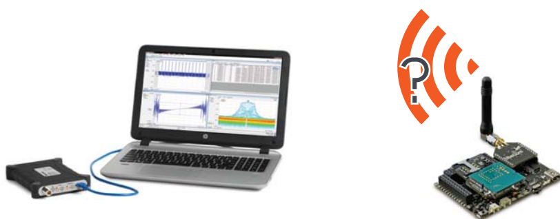
Figure 2. Tektronix RSA306B Real Time Signal Analyzer monitoring an IoT device.
