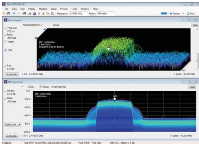
Figure 3-1. Spectrogram display, showing a waterfall plot of spectra as a function of time for an OFDM signal, compared to a DPX spectrogram in the bottom frame.
