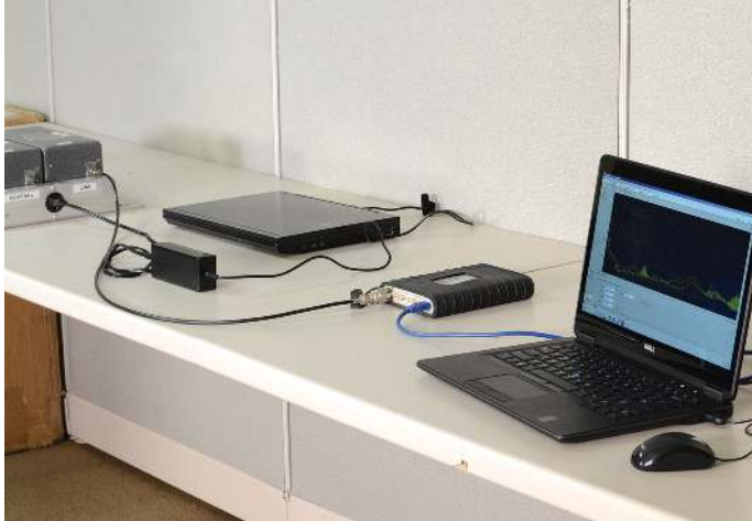
Figure 13. Basic pre-compliance conducted emissions test setup.
