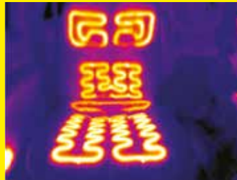
Figure 2. Production testing of car seat heater elements
