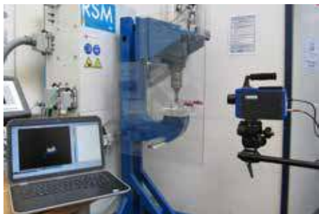
Thermal measurement of Friction Element Welding (FEW) process (passive thermography), Source: LWF
