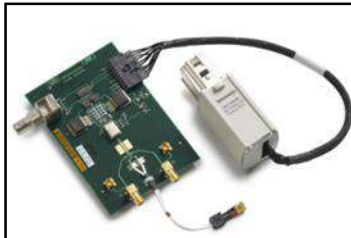
DC Calibration Fixture Use this fixture to calibrate your probes DC accuracy when making critical measurements.
