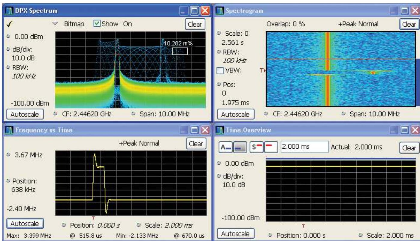
**Figure 38.** The analyzer triggered when the density in the DPX measurement box exceeded the threshold set by Trigger On This. You can see in the Spectrogram and Frequency-vs-Time displays that the signal event which caused the trigger was a quick frequency hop. The Time Overview shows that the signal amplitude never changed, so a power level trigger would not have worked.
