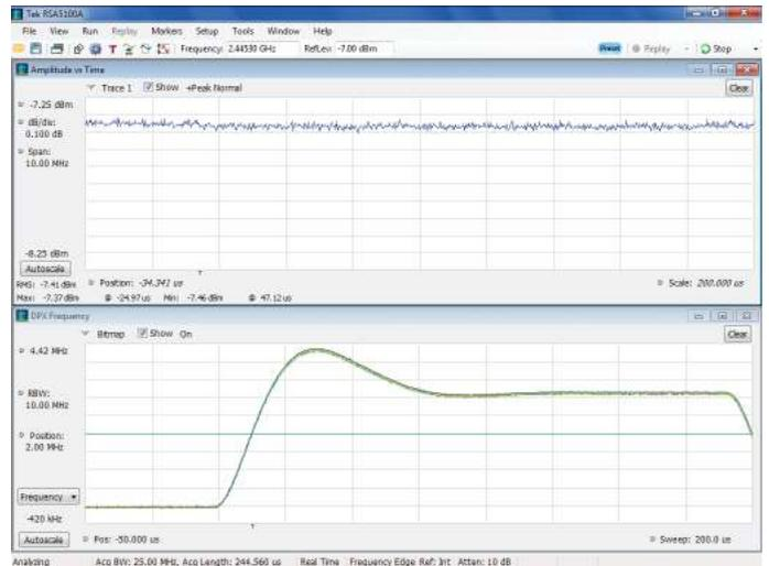
**Figure 40.** A frequency transition from a PLL circuit is recorded, using the Frequency Edge Trigger to capture the center of the transition point. In the lower display, frequency vs. time is displayed, and the line at the center of the display is the Frequency Edge trigger level. The upper display is amplitude vs. time with a vertical scale of 0.1 dB/division, showing that there is no amplitude transient on which to trigger.
