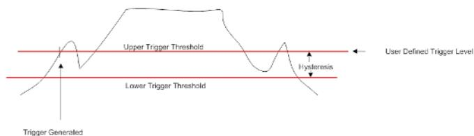
**Figure 41.** Hysteresis is applied to the frequency edge trigger to reduce the number of false triggers that result from noise signals. Starting from a user defined trigger level, hysteresis is subtracted from the user defined trigger level. The signal must pass through both the trigger level and the hysteresis level for a trigger to occur.
