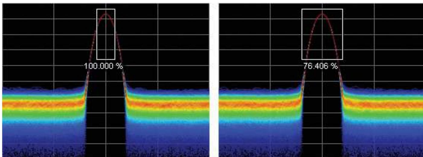
**Figure 31.** Density of signals defined within an area. Left: Correct measurement of a CW signal. All columns in the box include the signal. Right: Incorrect analysis window. The measurement is accurate, but probably not what you expected. Some columns in the box contain no hits, so they contribute zeros to the calculation of average density.
