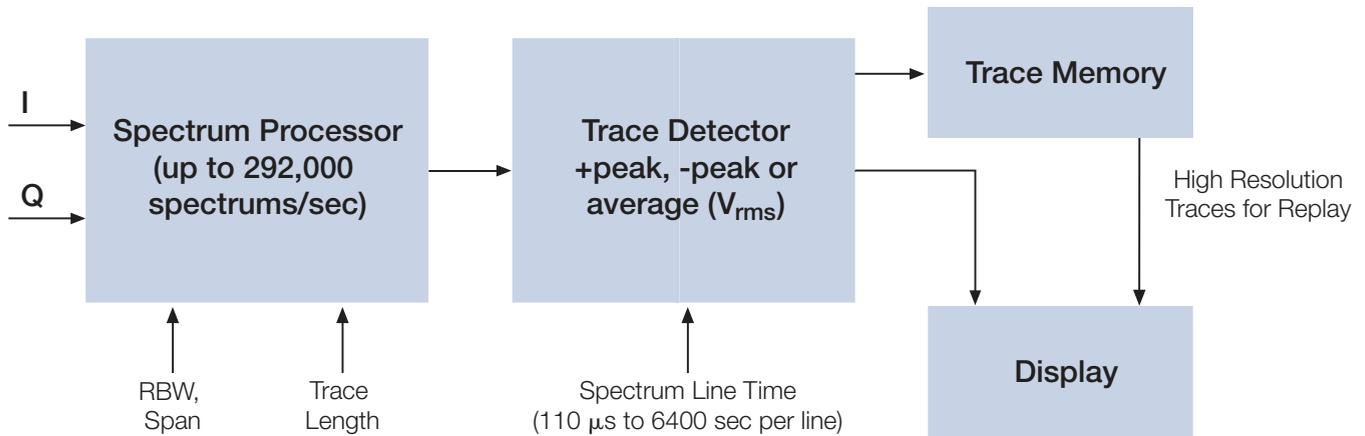
Figure 19. Block diagram of DPX Spectrogram processing.
