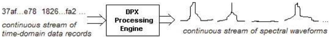
Figure 5c. Data records are processed in DPX transform engine.
