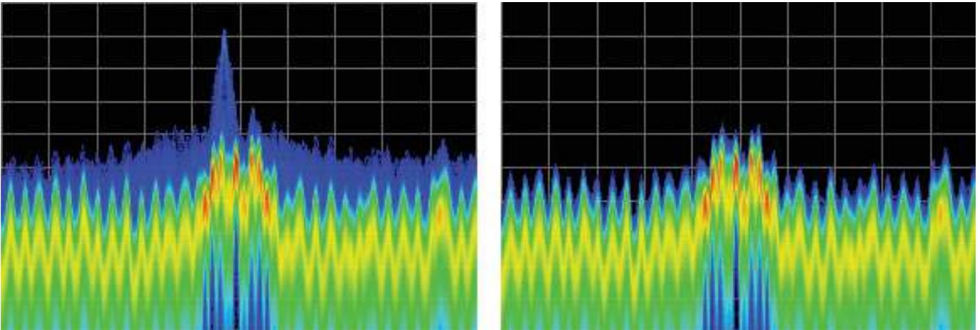
**Figure 33.** Example of fast transient discovery with and without variable persistence turned on. The display on the left, with variable persistence of 10 seconds, the occasional sub-second transient that spikes up above the normal signals is held in the display rather than disappearing as soon as the signal goes away. The display on the right, with persistence turned off, you have to watch the display continually to see the brief signal.
