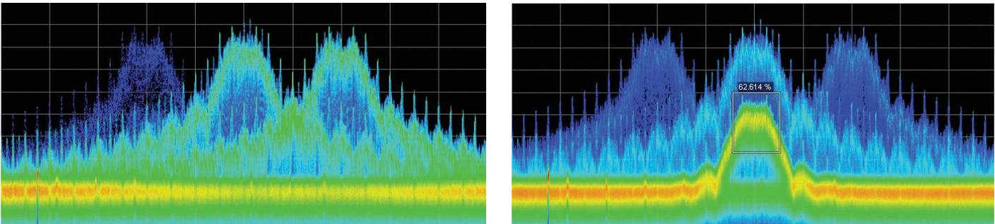
**Figure 37.** Example of Density Trigger Function. Left: A free-run DPX spectrum display showing pulses with varying frequency. Occasionally, a short pulse in the middle appears for a split instant, but it is hard to capture it with just a Run/Stop button. Right: The triggered DPX display shows the low-amplitude pulse that was not apparent in the untriggered display. The analyzer was set to trigger whenever the average density in the user-drawn box measured 50% or higher.
