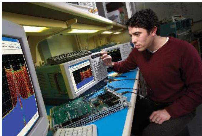
**Figure 43.** DPX spectrum display offers an intuitive live color view of signal transients changing over time in the frequency domain, giving you immediate confidence in the stability of your design, or instantly displaying a fault when it occurs.
