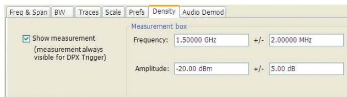
**Figure 32.** DPX Density control panel is used to define the area of interest for DPX density measurements.
