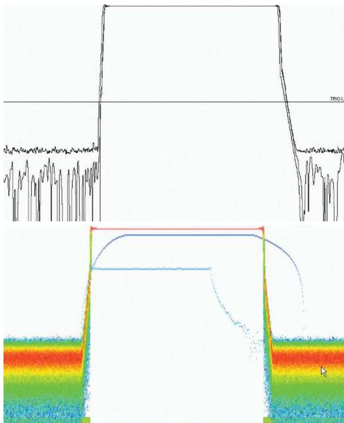
**Figure 24.** In this figure, conventional amplitude vs. time (Zero Span) on a spectrum analyzer is compared to DPX Zero Span. The signal contains three components, two of which occur very infrequently. In the same way that DPX spectrum illuminates elusive signals in the frequency domain, DPX Zero Span captures time domain signals at rates that are orders of magnitude faster than conventional signal analyzers.
