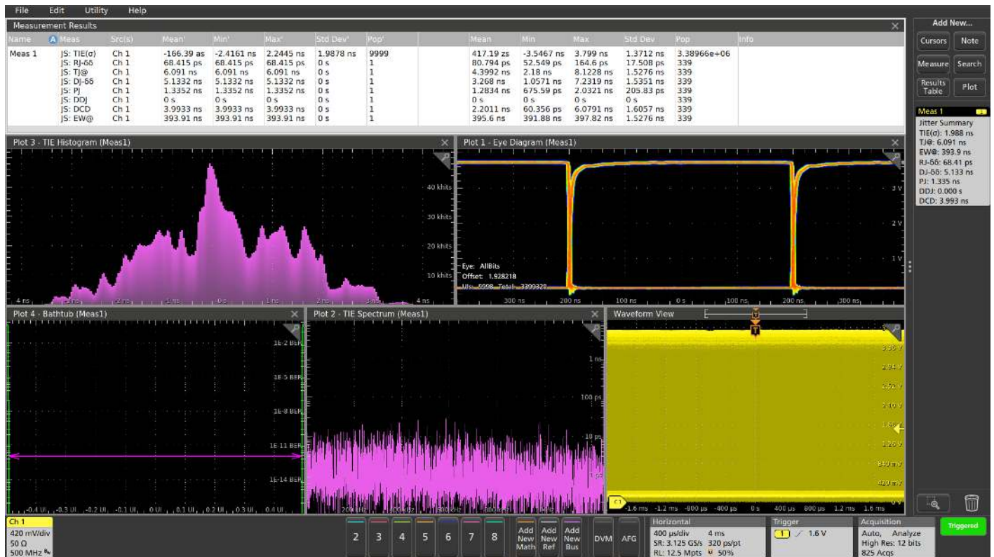
FIGURE 4. The 5 Series MSO Jitter Summary analysis of a 1.25 MHz clock.
