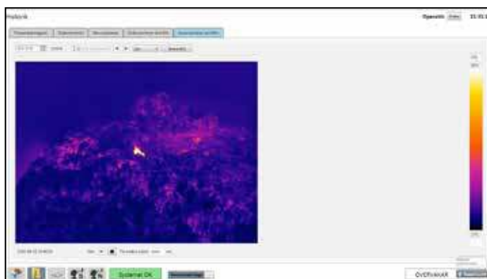
Claes Nelsson, Termisk Systemteknik: "TST Fire makes an accurate, real-time analysis of the FLIR thermal video image. If unusually high temperatures are detected, an alarm is triggered."
