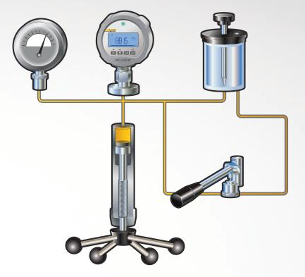
STEP 1 The pressure gauge should be mounted in the same orientation (vertical or horizontal) as in the process. An angle adapter such as the P5543 may be used.
