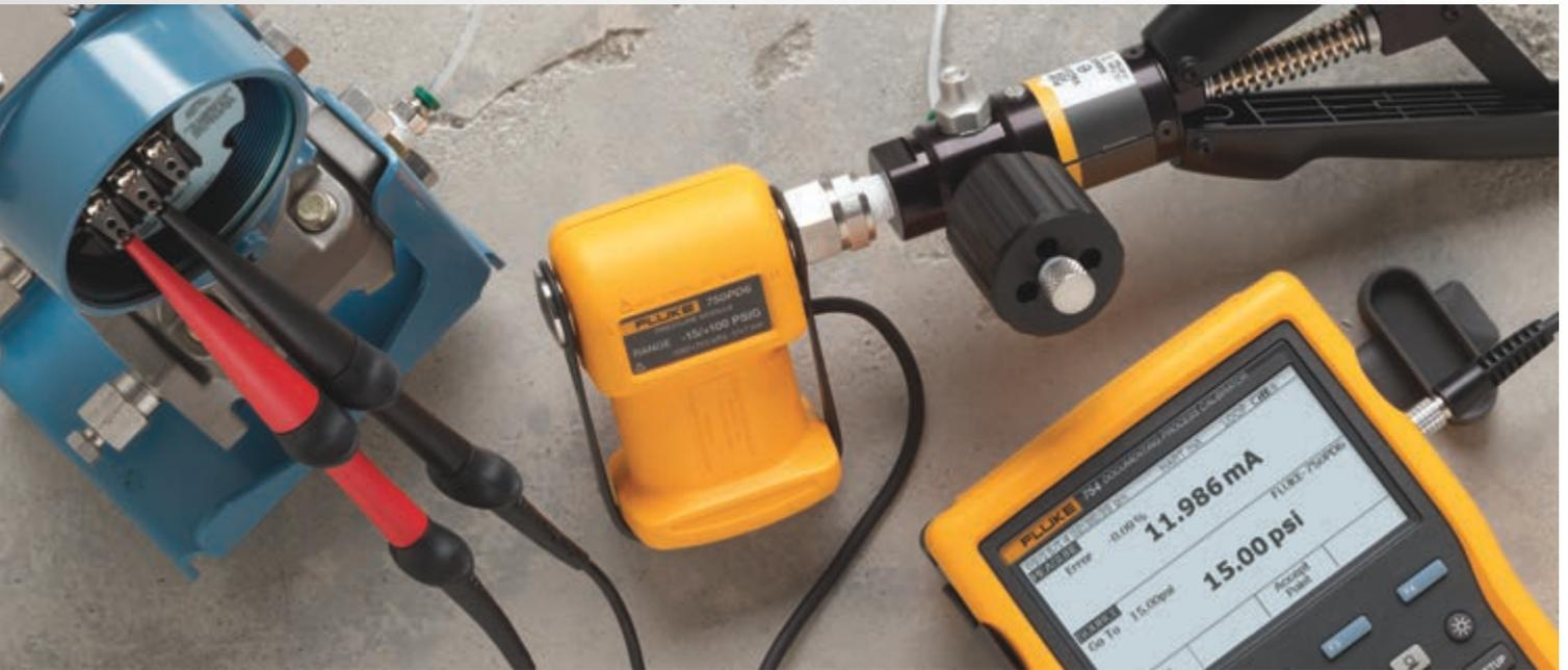
Classic methods for pressure switch testing have been superseded with the introduction of new pressure test tools. Today most pressure switches are tested with a pressure gauge mounted to a pump to supply and measure pressure, and a DMM set to continuity to verify the opening and closing of the switch. The technician or electrician making the test is required to interpret the pressure applied to the switch
