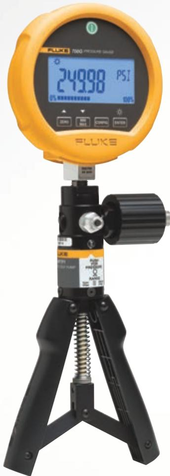
It's important to select the proper pump and gauge to match the testing application at hand—a good guideline is the testing device should be 4-10 times more accurate than the device being tested. To achieve this, match the measurement to be made as closely to the full scale value of the test gauge. This delivers the best accuracy from the gauge.
