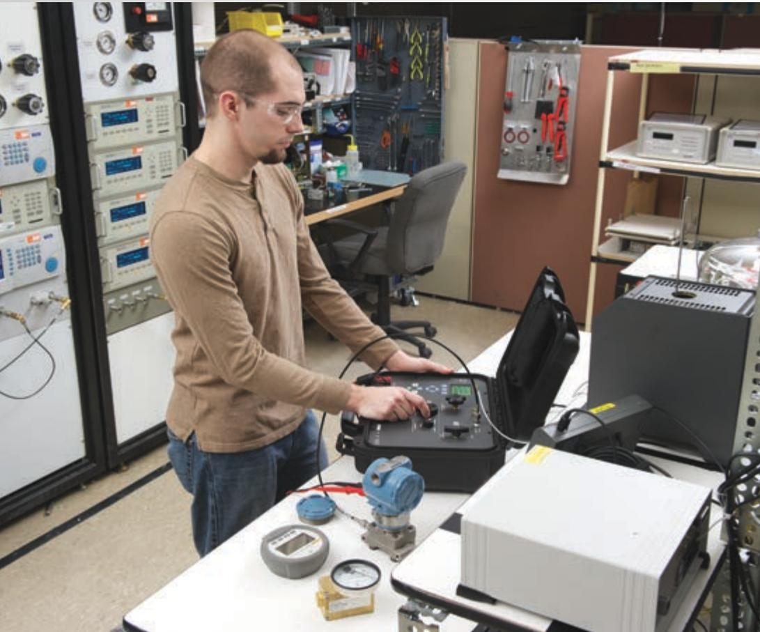
Technicians calibrate at the bench to ensure calibrations are effective and don't result in degradation of performance. They ensure that all components are in good working order prior to installation, and can evaluate them when component failure is suspected. The bench provides a stable ambient environment for calibration, an opportunity to use the most accurate equipment, and protection from factory conditions during the commissioning, testing, and calibration of pressure transmitters.
