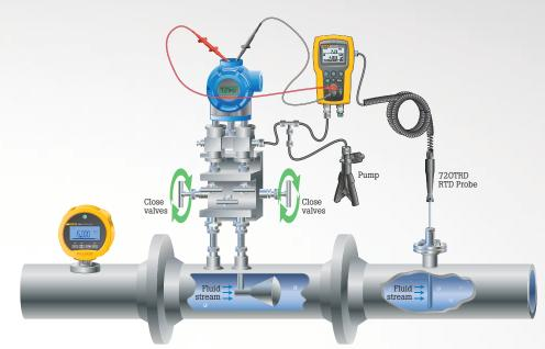
To get started, isolate the flow computer from the pipeline. It is normally installed with a 5 valve manifold. If so, closing the valves on the pipeline side of the manifold should isolate it. Be sure to follow local policy and safety procedures when performing this isolation step. Set the P1 sensor of the 721 to measure inH2O and the P2 sensor to measure PSI and the temperature sensor to measure degrees Celsius or Fahrenheit as needed.
