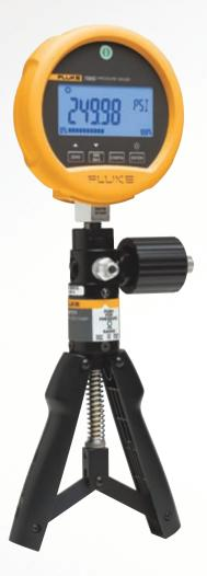
It's important to select the proper pump and gauge to match the testing application at hand—a good guideline is the testing device should be 4-10 times more accurate than the device being tested. To achieve this, match the measurement to be made as closely to the full scale value of the test gauge. This delivers the best accuracy from the gauge.
