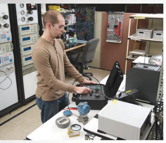
Technicians calibrate at the bench to ensure calibrations are effective and don't result in degradation of performance. They ensure that all components are in good working order prior to installation, and can evaluate them when component failure is suspected. The bench provides a stable ambient environment for calibration, an opportunity to use the most accurate equipment, and protection from factory conditions during the commissioning, testing, and calibration of pressure transmitters.
