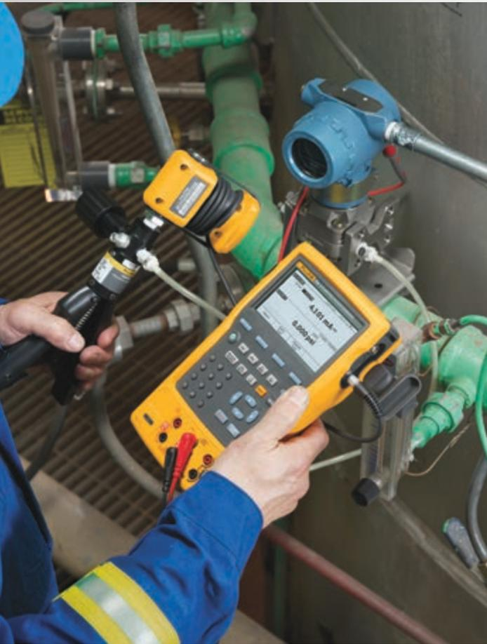
Pressure transmitter manufacturers have improved the accuracy and technology designed into these smart pressure measurement devices. Many conventional calibration tools have become inadequate or simply unable to test and calibrate these high accuracy pressure transmitters. Better test solutions are required.
