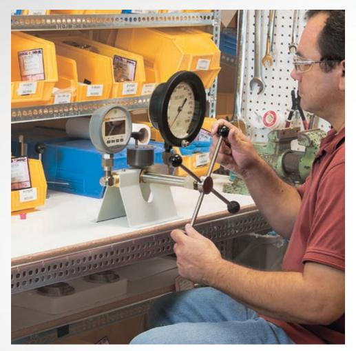
A pressure comparator is a convenient instrument for bench pressure calibration. Bench calibrations are performed to maintain reference conditions and to obtain the lowest possible uncertainties. The bench is also a convenient place to inspect, adjust, and repair the devices under test.
