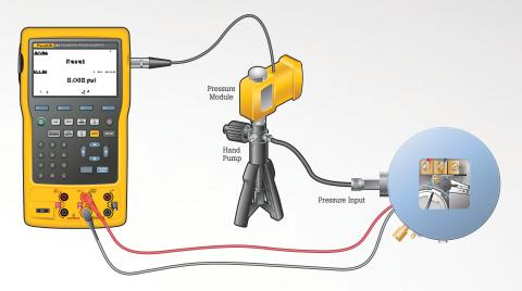
With a modern documenting calibrator you can test for dry contacts opening and closing on the switch or if you are using the Fluke 753 or 754 you can leave the switch connected to the live voltage and the calibrator will measure the changing AC voltage and interpret it as opening and closing of the switch.
