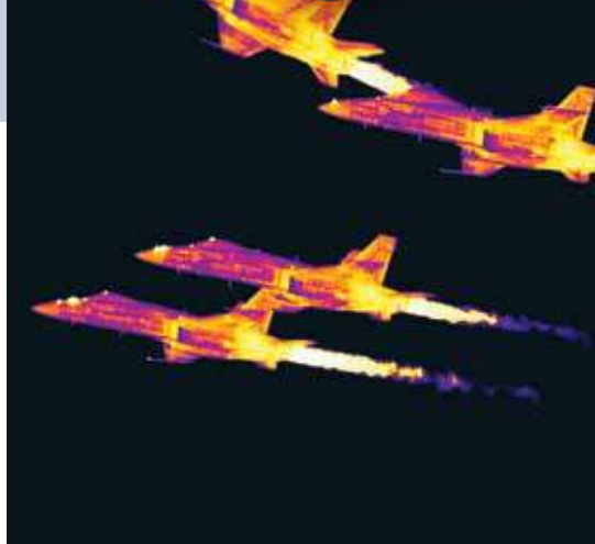
Stop motion image of FA-18 Hornets from a FLIR InSb cooled thermal camera
