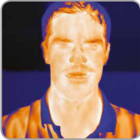
Figure 12. IR image from a 1024 × 1024 InSb detector camera
