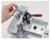
Pull the lock lever toward you to allow the probes to be lowered. This design keeps the probes from being lowered inadvertently.
