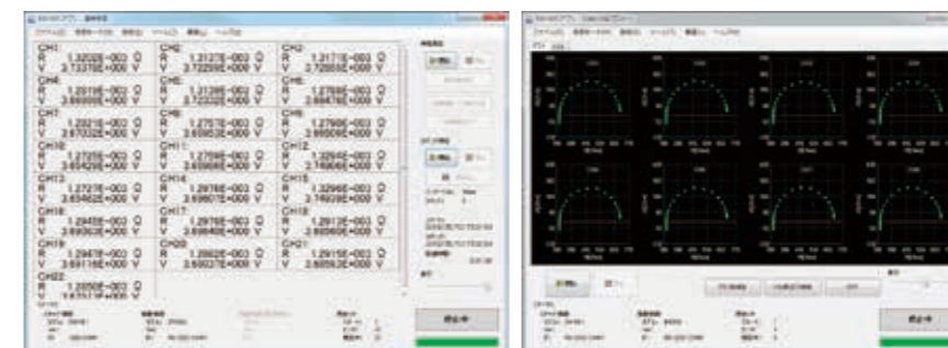
Logging function (Interval setting: 1 second to 60 minutes)
